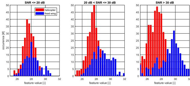
Fig. 6. Histogram for the micro-Doppler spectrum periodicity feature plotted for different SNR, left:  $SNR \leq 20$  dB, middle:  $20 < SNR \leq 30$  dB, and right:  $SNR > 30$  dB.
