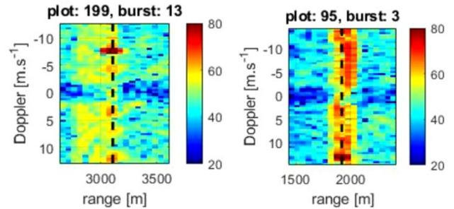
Fig. 3. Range-Doppler representation of a helicopter measurement (left) and a fixed-wing aircraft measurement (right). The colour scale is in dB.
