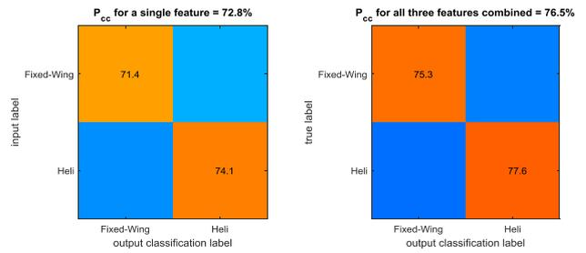
Fig. 8. Confusion matrices for single bursts achieved with one single feature (left panel) and with the micro-Doppler features combined (right panel).
