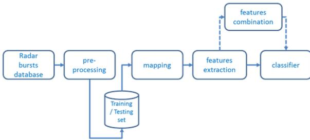
Fig. 4. The radar component's training/testing classification chain.
