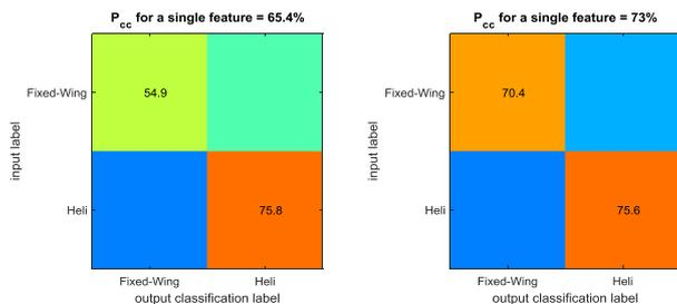
Fig. 7. Confusion matrices for single bursts for the maximum observable micro-Doppler speed feature for a classifier that does not take SNR into account (left panel) and a classifier with SNR dependency included (right panel).
